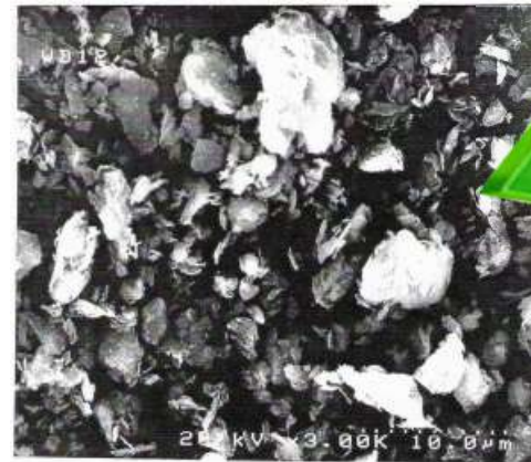
Micropores in porous ceramic raw materials Electron micrograph × 5,000 magnification
