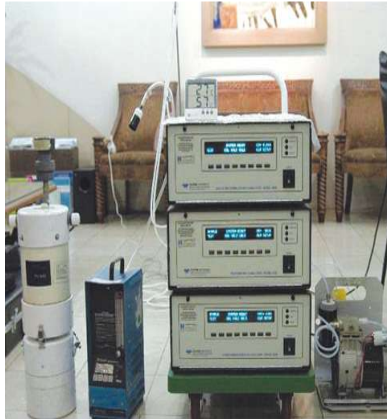
Measurement of indoor pollutant (CO,NO2,Ozone,Asbestos)
